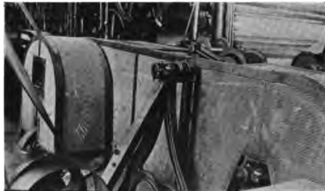
Fig. 5. Enclosure of Core Wheel, etc.* Fig. 5 shows a neat guard of woven wire construction.
